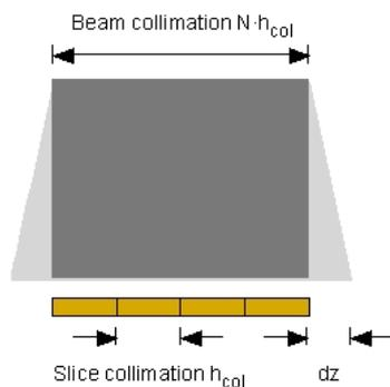
**Fig. 1** Dose profile free-in-air for a quad-slice scanner (dark grey: umbra, light grey: penumbra); overbeaming is characterized by the parameter  $dz$ .
