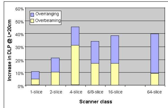
**Fig. 3** The percentage increase in DLP from the combination of overbeaming and overranging effects, for 20 cm scan length and parameter settings that are typical for each scanner class.
