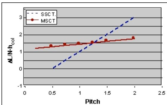
**Fig. 2** Overranging characteristics of typical single- (SSCT) and multi-slice (MSCT) scanners.
